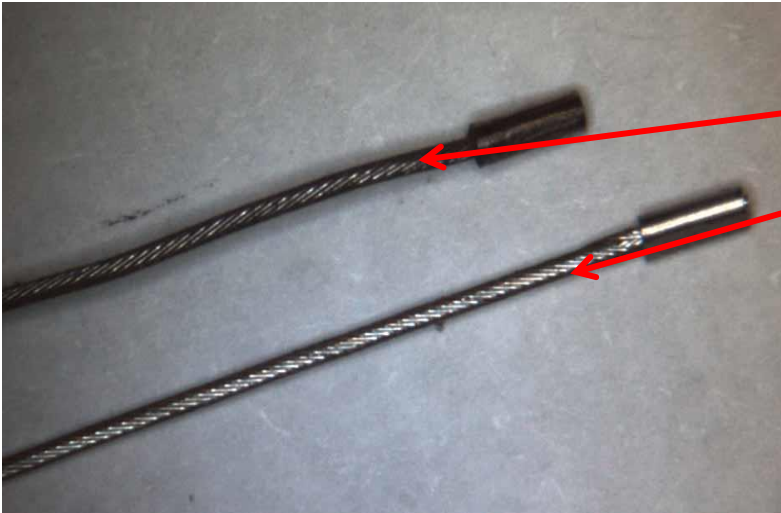
Corroded articulation wire Common cause: Fluid ingress Good articulation wire
