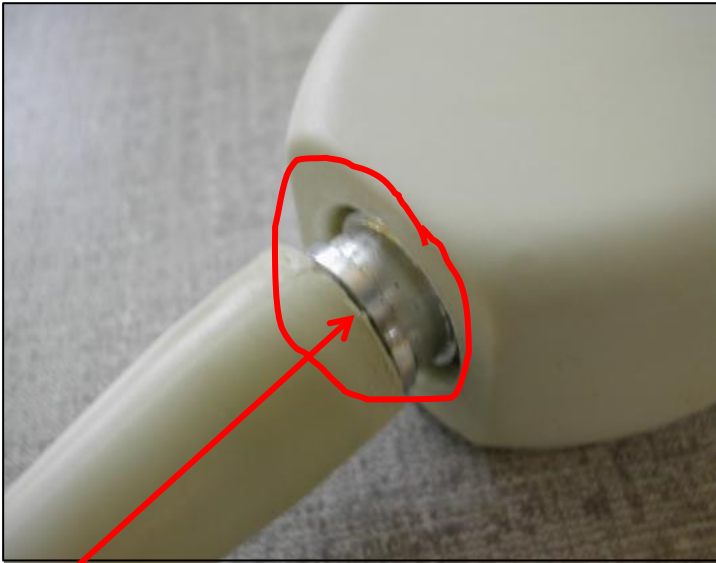
Strain relief pulling away from array housing
