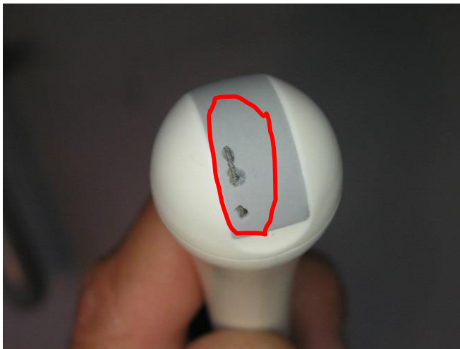
Hole in Lens Common Cause: Rough cleaning
