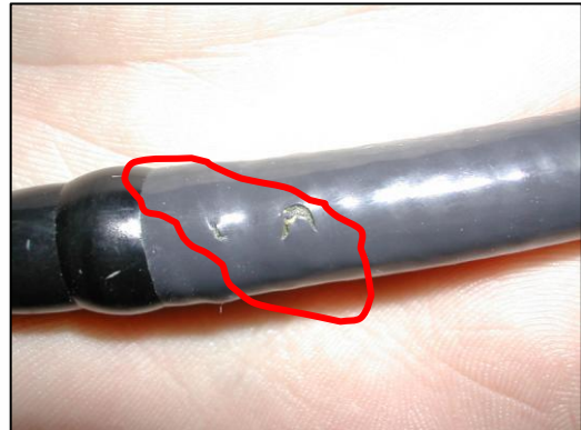
Holes in bending rubber Common cause: Bite guard not used
