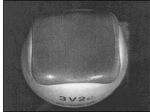
Swollen Lens Common Cause: Manufacturing defect
