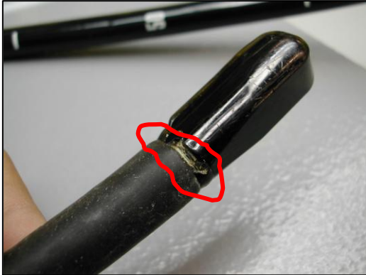
Broken seal near head of TEE probe Common cause: Rough handling, poor storage, or aggressive cleaning
