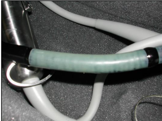
Contaminated bending rubber Common Cause: over-soaking in Cidex
