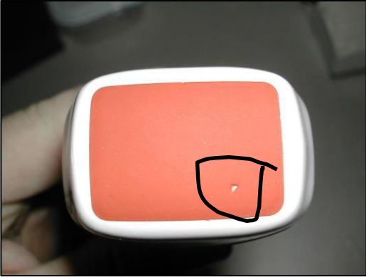
Hole in Lens Common Cause: Rough cleaning
