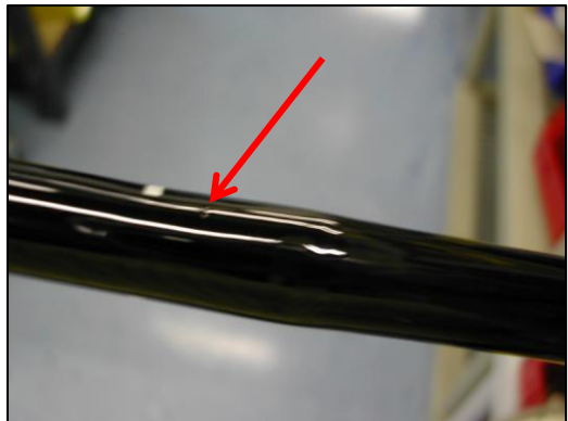
Bite mark in bending rubber Common cause: Bite guard not used
