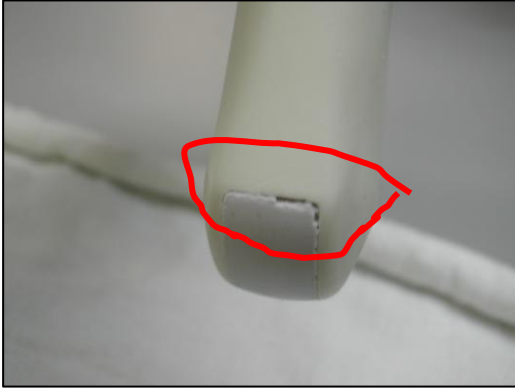
Lens separating from housing Common Cause: Over cleaning and use of inappropriate cleaning agents.
