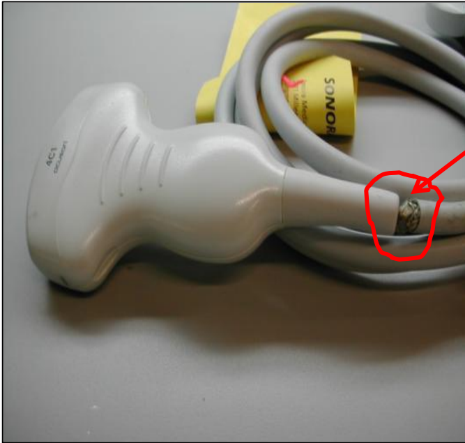
Cable pulled out from under strain Common cause: Pulling the system by the probe
