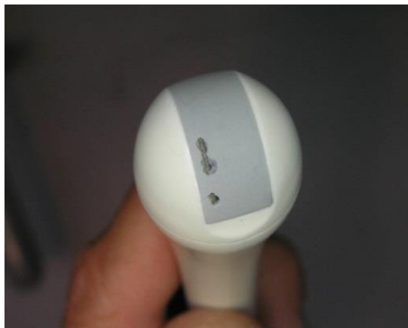
Photo 1 Multiple Holes in Lens
