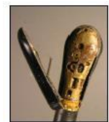
Photo 4 Fluid Ingress and the Damage Done
