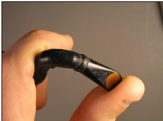
Photo 5 Insertion Tube Sleeve Damage
